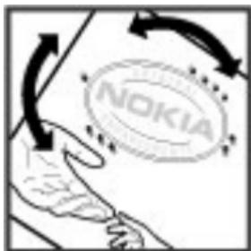
Successful completion of the steps is not a total assurance of the authenticity of the battery. If you cannot confirm authenticity or if you have any reason to believe that your Nokia battery with the hologram on the label is not an authentic Nokia battery, you should refrain from using it, and take it to the nearest Nokia authorized service center or dealer for assistance.
