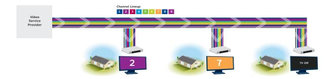
In the traditional cable TV or satellite network – using broadcast radio frequency (RF) video technology – all content constantly flows downstream to each customer, and the customer switches the content at the settop box. The customer can select from among as many choices as the cable or satellite company can fit into the "pipe" flowing into the home. The broadcast network is one-way.
