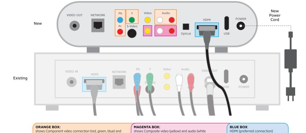
**Note:** if using coaxial connection, apply sufficient force to tighten the connectors past "finger tight." Failure to properly tighten this connection will degrade the signal and can cause intermittent or continuous video problems.
