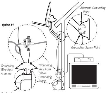
Cold water pipe only Use grounding wires #10 copper or #8 aluminum
