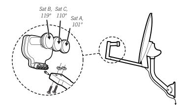
Hooking up cables (one shown) to the LNB and attaching the LNB to Antenna — up to four cables can be connected this way.
