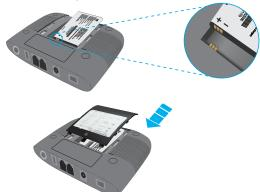
**NOTE**: The battery must be installed at all times for your Wireless Home Phone device to operate properly, even when plugged into a power source. It may take five (5) hours to fully charge (battery will charge inside the device while connected to a power supply).
