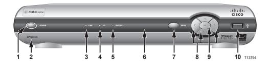
1 Power Turns the receiver on or places it in standby. To restart the receiver,
