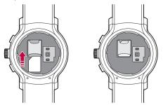
4 Close the SIM card cover using the SIM card cover opener as shown below. Align the SIM card cover opener with the holes located on the back of the watch, then turn the cover clockwise.
