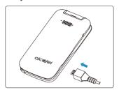
Insert the small end of the charging cable into the charge port as shown and connect the charger to a power outlet.
