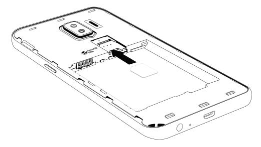
2. Slide the memory card into the slot with the gold contacts facing down.
