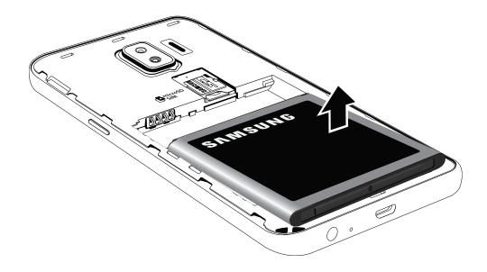
Remove the battery from the device.
