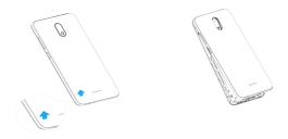
2. Remove the battery via the notch under the right bottom edge of the battery.
