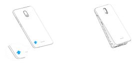
2. Insert the battery by aligning the gold contacts of the battery with the contacts in the phone, and gently press the battery down into place.
