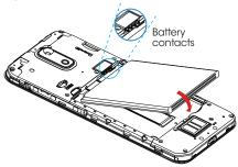
Reattach the back cover and press firmly around sides and all four corners until it snaps into place.
