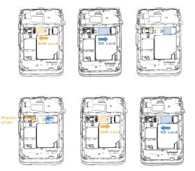
To insert a Nano SIM or microSD card, push the Nano SIM or microSD card into the corresponding card slot with the gold-connectors facing down. To remove the Nano SIM or microSD card, push down on the plastic clip and pull the Nano SIM or microSD card out.
