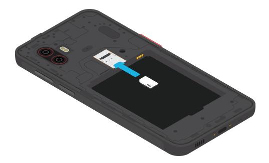
4. Slide the microSD card into the slot with the gold contacts facing down.
