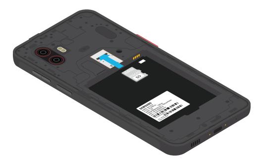
5. Insert the battery into the opening on the back of the device, making sure the connectors align. Gently press down to secure the battery.
