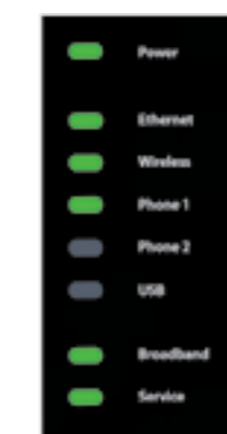
Wi-Fi Gateway indicator lights
