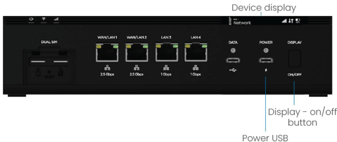
2. Wait for the router to power on. This can take up to three minutes. You'll know it's powered on when the device display shows your cellular network name and arrows indicating traffic is active.
