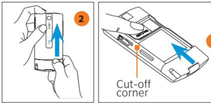
Note: To remove the SIM card, press down the tab in front of the SIM card slot opening with one finger, and slide the SIM card out from the slot with another finger.
