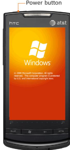
It may take several minutes for the TouchFLO 3D interface to load during initial setup. Do not press any buttons or turn off the device until the device completes the startup.
