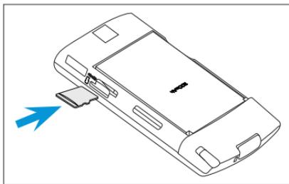
Note: To remove the microSD card, press it to eject it from the slot.
