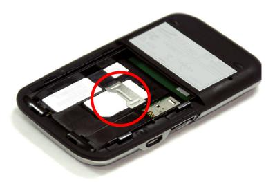
Insert the battery, lining up the contact points as shown, and then replace the door.
