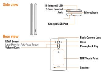
**LDAF Sensor (Laser Detection AutoFocus Sensor):** This sensor measures the distance to the subject using laser technology and allows for improved focusing speed and object detection in low-light situations.
