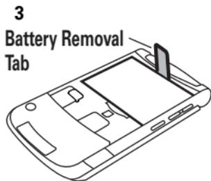
Make sure that the **Battery Removal Tab** sticks out from under the battery.
