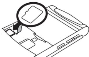
To **remove the memory card**, lift up the rubber grommet and slide the card back out of the holder.
