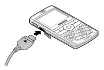
**Note:** The following illustration shows the **correct** and **incorrect** method for connecting the charger. Verify the arrow on the adapter is showing and pointing to the handset for a correct connection. If it is not, damage to the accessory port will occur therefore voiding the phones warranty.
