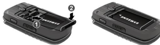
3. With the battery in position on the phone, place the cover back on the handset and turn the grooved dial clockwise until the cover locks.
