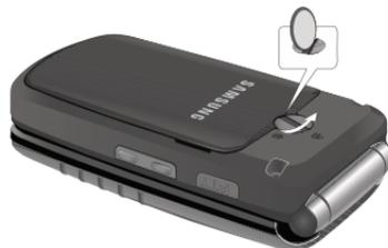
2. Use the grooves at the top of the cover to lift the cover up and away from the back of the phone.
