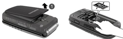
**Warning:** Please note the printed circuit side faces down when inserting the card.
