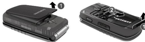
3. Lift the battery up and away from the phone, as shown.
