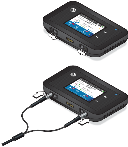
Figure 4. External antennas with TS-9 connectors
